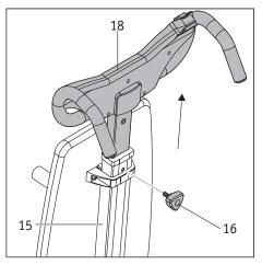
• Loosen and remove the upper adjustment knob [16] and pull then handlebar [18] from the standpipe [15].
