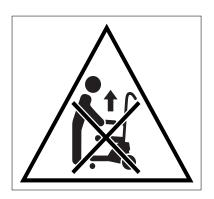
Do not use armrests to lift the device, especially if the person to be conveyed is sitting in the scalacombi. To ensure user-friendliness, the armrests are rotatable and detachable (e.g. for transfer to the seat of the scalacombi) and might be inadvertently pulled off, depending on direction of force.
