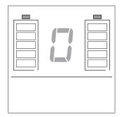
Push the button [24] on the remote control to simultaneously switch off both e-motion wheels. A zero and the charge status of both battery packs is indicated in the display. A beep sounds at the e-motion wheels.
