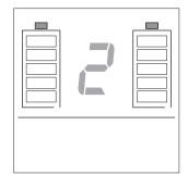
Push the button [22] on the remote control to simultaneously switch on both e-motion wheels in power stage 2.
