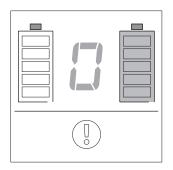
If an error is indicated according to the table on the following page and the right battery symbol flashes at the same time, the error indicated occurs only in the right wheel or in the battery pack of the right wheel.
