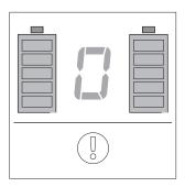
If an error is indicated according to the table on the following page and both battery symbols flash at the same time, the error indicated occurs in both wheels or in the battery packs of both wheels.
