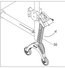
• Once the wheels have been attached, you can return the anti-tippers to the original position. To do so, push the wheelchair forward and the holding rod [30] back with the foot at the same time.
