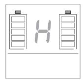
If button 1 or 2 is pressed longer than 3 second to activate or deactivate the rollback lock, a long signal tone sounds on the e-motion wheel in each case. If the rollback lock is active, the following will be displayed: the current charge status of the two battery packs, an "H" in alternating fashion, the power stage currently set (1 or 2) and, if applicable, additional functions (e.g. the button lock). In case of an error, only the corresponding error code is displayed.
