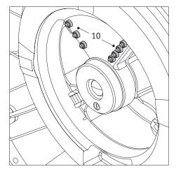
Carry out the following steps to insert a battery pack again in the wheel hub:
