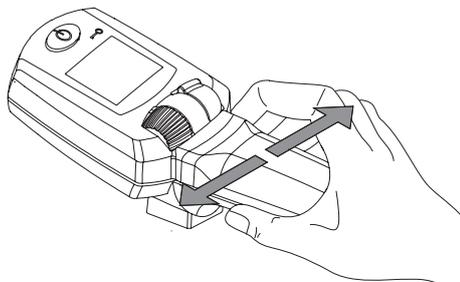
The electronics in the handle register the movements made by the user's hand. A slight deflection of the lever to the left or the right is converted into a travel command for the e-fix wheels so that you can navigate bends without a great deal of effort.
