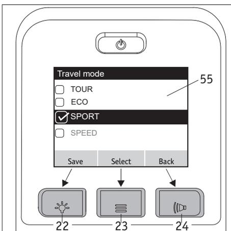
The control unit buttons are assigned to the menus and sub menus as follows:
