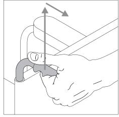
• Whilst doing so, pull the wheelchair upwards and to the rear a little by its handles until the wheelchair has been raised and the anti-tippers click into a fixed position.
