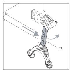
• Once the wheels are fitted, you can return the anti-tippers to their starting position. To do this, push the wheelchair forwards and push back the holding rod [21] using your foot at the same time.
