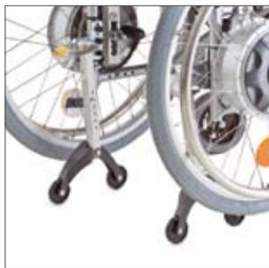
**Anti-tippers with jack-up function:** This makes it even easier to remove the e-fix wheels.
